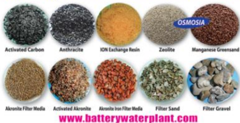
Figure 4.5 Media used for specific contaminant removal, from: http://batterywaterplant.com/images/iron_removal_chemicals.jpg
